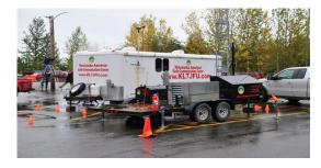
We have a Mobile Communications Unit with VHF, UHF HF and Public Safety and other radio services capabilities. As a compliment to this trailer we have also constructed a support trailer carrying a crank-up tower and generator. This will make it possible for MARA to go to most locations and operate under any conditions on all bands. We have portable GO-KITS to allow for deploying to different locations.
